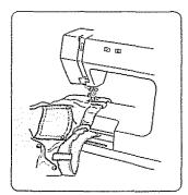
Bar tacking to reinforce pockets, plackets and waistlines on readymade or home-made garments to avoid fabric bunching around the needle.
